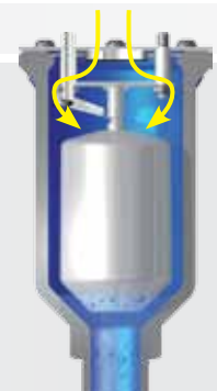
Admission of large quantities of air during the emptying
