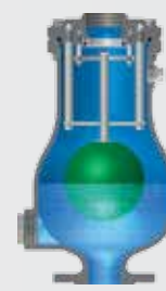
Admission of large quantities of air during the emptying
