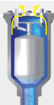
Evacuation of large quantities of air during the filling
