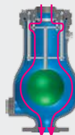
Purge of air during operation
